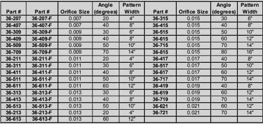
Note: Carbide tips spray pattern is guaranteed to +/- 5 degrees (one inch). Double degrees to determine fan inches.
