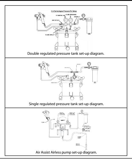
NOTE: When setting up a spray gun for spraying a specific material, it is recommended to use the lowest possible pressure settings to achieve the desired results. Excessive fluid and air pressures result in premature nozzle replacement, greater overspray, and more frequent booth filter replacement.
