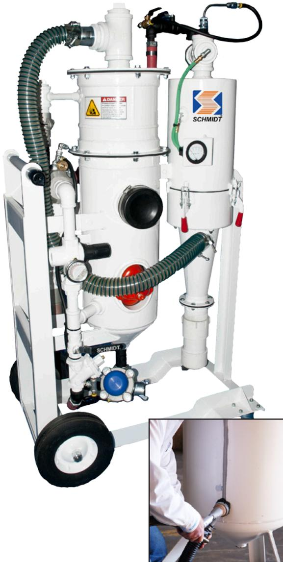
The Schmidt miniBRS is a compact and easily maneuverable abrasive blasting system that blasts and then recovers spent abrasive, contaminants and dust in the same step, eliminating the need for containment. The system can also be used to blast and then vacuum abrasive independently.
