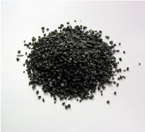
Coal Slag is a relatively fast cutting angular media that provides surfaces with ideal anchor patterns. Typical usages include the removal of heavy rust, tank linings, mill scale and most thick coatings. Coal Slag's are used on ships, barges, bridges, tanks and etc. It is not considered a recyclable abrasive, but it offsets the lack of recycles with its low purchase cost.
