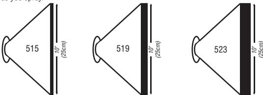
**Different fan width - same orifice sizes:** The example below demonstrates the difference between tips with the same orifice size, but increasing fan sizes. The same amount of coatings is applied over a larger area - or less coating per square inch using the same pressure and hand-speed as you spray. When necessary, remember to size up or down your orifice as you size up or down your fan width if you want to apply the same amount of coating per square inch.
