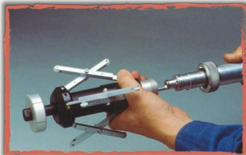
Orbiter I coats 3.5-inch through 7-inch pipes.
