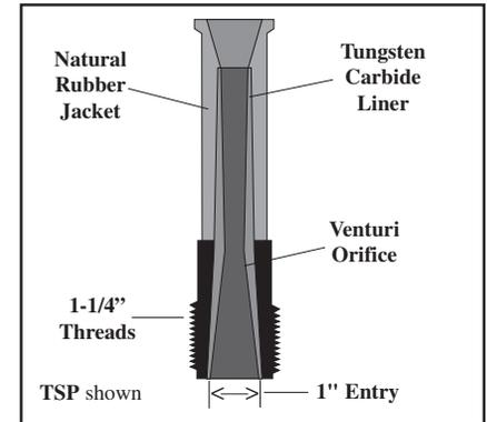
With all related equipment correctly assembled and tested, the operator points the nozzle toward the surface to be cleaned and presses the remote control handle to begin blasting. The operator holds the nozzle and moves it smoothly at a rate that produces the desired cleanliness. Each pass should overlap slightly.
